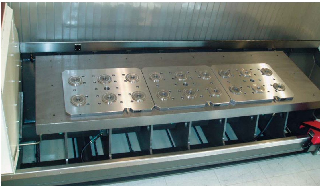
3 Zeropoint Quickclamping Stations fixed on a machining center
